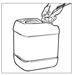
Place the siphon tube firmly in the opening of the free-standing container (pay attention to colour coding).
